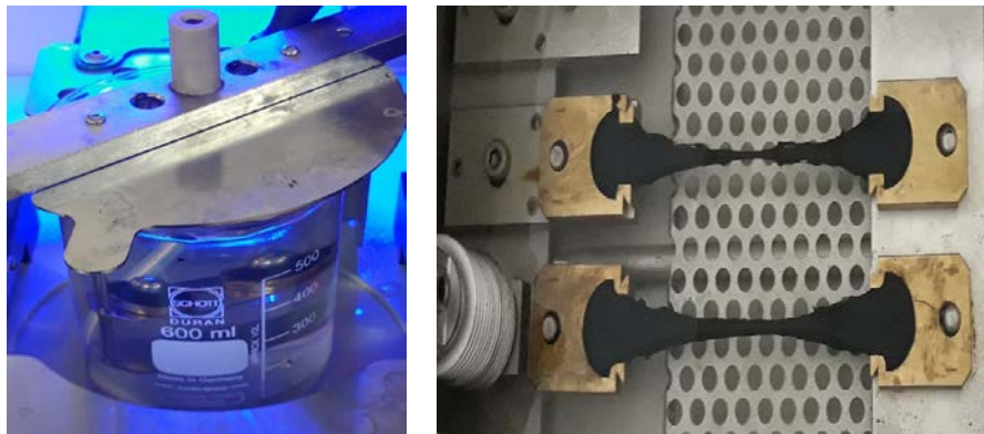
Figure 3: Testing process: a) ring and ball ; and b) ductilometer.
